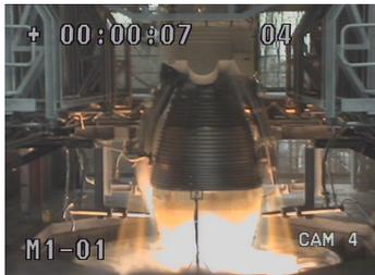
This is a version of the Ariane 5 Vulcain® 2 engine especially adapted for the Ariane 6 main stage, to simplify production and to lower costs. To reach these objectives the engine integrates technologies such as a gas generator built using 3D printing, a simplified divergent nozzle, and an oxygen heater for tank pressurization. These adaptations contribute to achieving the cost targets set for the Ariane 6 launcher, while retaining the efficiency and reliability demonstrated on Ariane 5.
