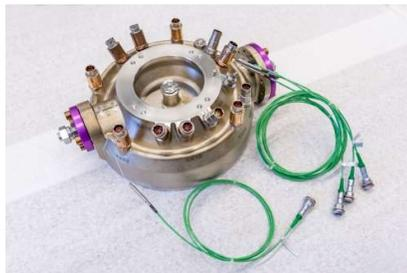
The current test configuration incorporates ArianeGroup's first full-scale 3D-printed injector head for next-generation thrust chamber assemblies. It has now successfully performed the first hot-fire tests in representative conditions on the German Aerospace Center (DLR) P3.2 test bench in Lampoldshausen. Drawing on experience from earlier, smaller-scale R&T activities, this single-piece injector head, made of Inconel 718, is the latest development step in the
