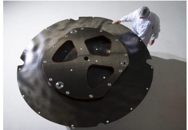
Ultra-light satellite antenna reflector.
