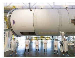
Ariane 6 liquid oxygen tank for combined tests (Les Mureaux)
